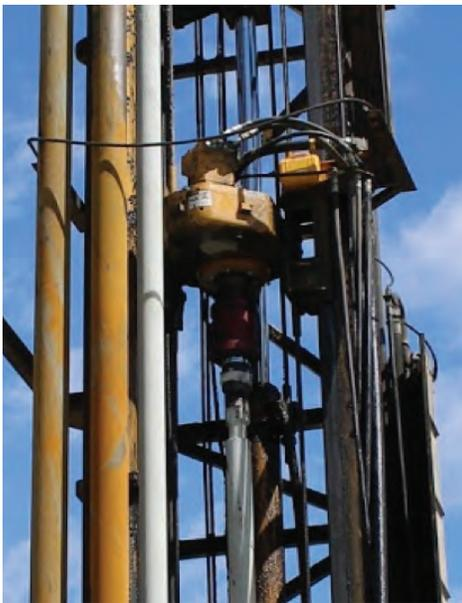
*RHINO™ from DataCloud mounts on the mast machinery. Seamless "set and forget" operability.*
